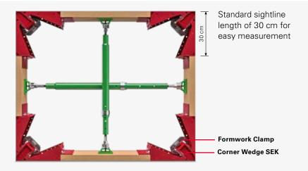
The VARIO Element VE is suitable for recesses in walls and slabs from 75 to 300 cm wide, as well as for door recesses of any width. The formlining thickness can be adjusted between 21 and 55 mm without requiring any tools.
